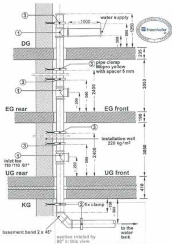
Figure 4 Installation plan of the pipe system "Ultra Silent 110 x 3.4" (manufacturer: HULIOT (A.C.S) LTD.), mounted with pipe clamps "Mupro yellow, with spacer 5 mm". Drawing not to scale, dimensions in mm.
